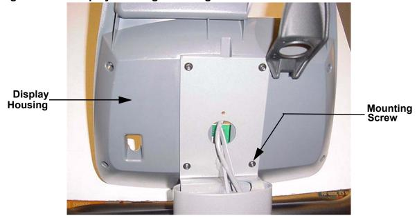
11. Set the display housing near the upper end of the replacement display column and feed the heart rate cable into the display housing and out of its access hole where the vertical handlebars will mount, See Diagram 7.9. Feed the data cable into the display column and out of its access hole as shown in Diagram 7.17.
